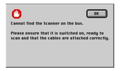
Firstly check that the scanner is switched on and that the USB cable is firmly seated into your MAC and scanner. We can use the Apple system profiler to confirm installation. Click the apple icon and select Apple System Profiler. Select the **Devices and Volumes** tab and check that the scanner is present. In this case USB1.
