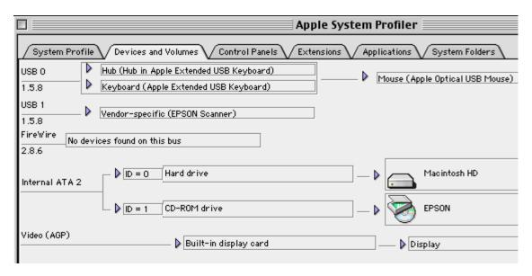
If the scanner is not here try the USB cable in a different port or a different USB cable. Also ensure that there is power to the scanner. If the scanner is apparent you need to reinstall the driver. Please click the link for instructions:
