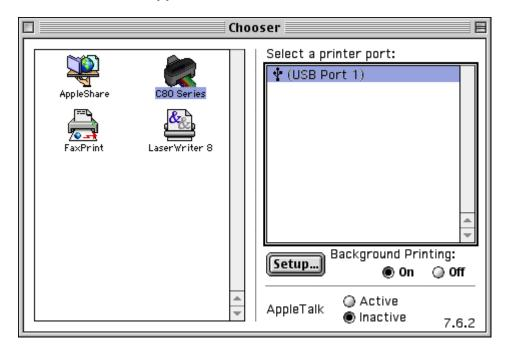
Your printer will need to be configured like the example above, with Background printing **on** and apple talk set to **inactive**. There must also be a valid port available, in this case **(USB Port 1)**. If there is not a valid port in the chooser ensure the printer is on and connected directly to the MAC.
