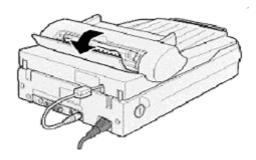
After the removal of the paper jam ensure that the ADF is seated correctly and the back cover is closed.
