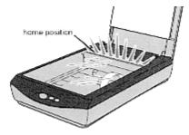
Disconnect the USB cable from the scanner. Disconnect the AC adapter and then slide the transportation lock left to the lock position. Unlock when desired for use.
