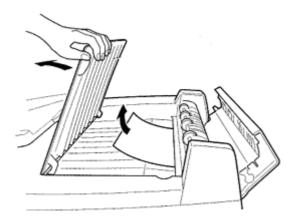
After removing the jammed paper, close the Automatic Document Feeder cover.
