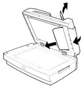
**Note**: Be careful not to pull too hard. If the paper tears, open the middle cover and remove the paper as shown as below.
