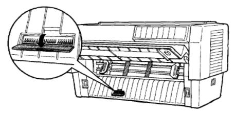
5. Use a pointed instrument, such as the tip of a ballpoint pen, to turn the switch either on or off. A DIP switch is on when it is up, and off when it is down.
