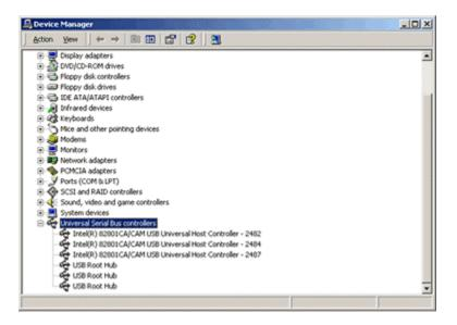
In this example the PC has an Intel 82801 CA/CAM Universal Host Controller. If the root hub is displayed with an exclamation point in a yellow circle, verify that the BIOS is assigning an interrupt request (IRQ) to the root USB controller. This is required for the device driver to be loaded.
