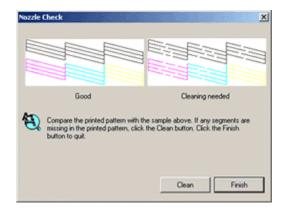
Repeat the process until the issue is resolved. If cleaning doesn't resolve the issue then it is recommended that you install a new set of cartridges.
